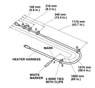
12. Plug the connector end of the heater harness into the engine block heater.
