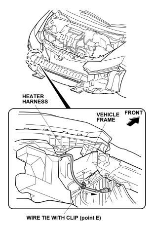
21. Secure the heater harness to the vehicle bracket with one black wire tie.
