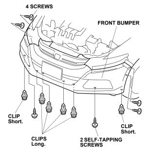
Release four retaining tabs on each side of the front bumper.
