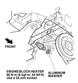
10. Secure the engine block heater bracket to the engine with one 6 x 12 mm washer-bolt.
